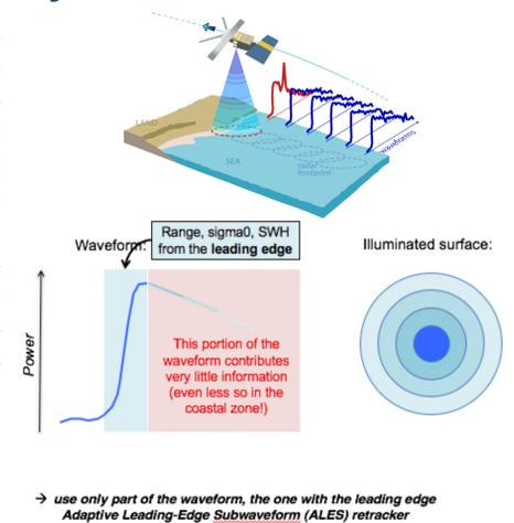
Figure 3. Principle of operation of the ALES altimeter coastal processor developed at NOC
